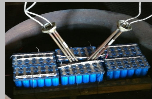
Electric heating coil TERMOWATT 3000W set-up
