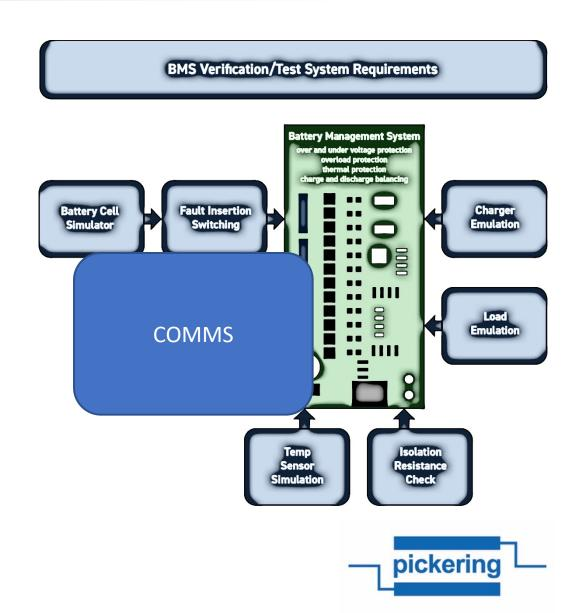
Flexible PXI-based BMS Test System Pickering Interfaces
