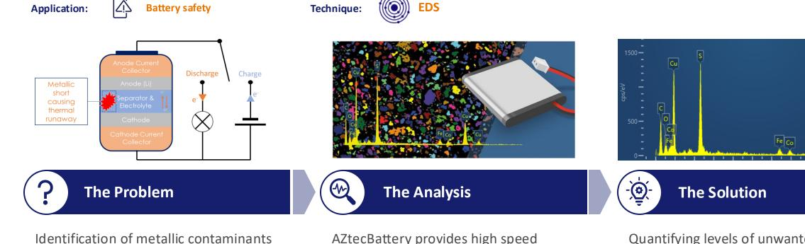
Identification of metallic contaminant introduced during the mining and subsequent manufacturing of Li-ion batteries can cause short circuits AZtecBattery provides high speed automated software analyses of EDS spectra identifying and classifying elements in contaminants and their morphology
