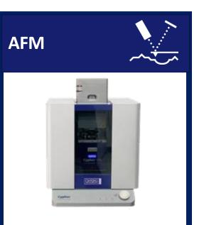
3D characterisation of surface nanoscale structure, mechanical and electrical properties
